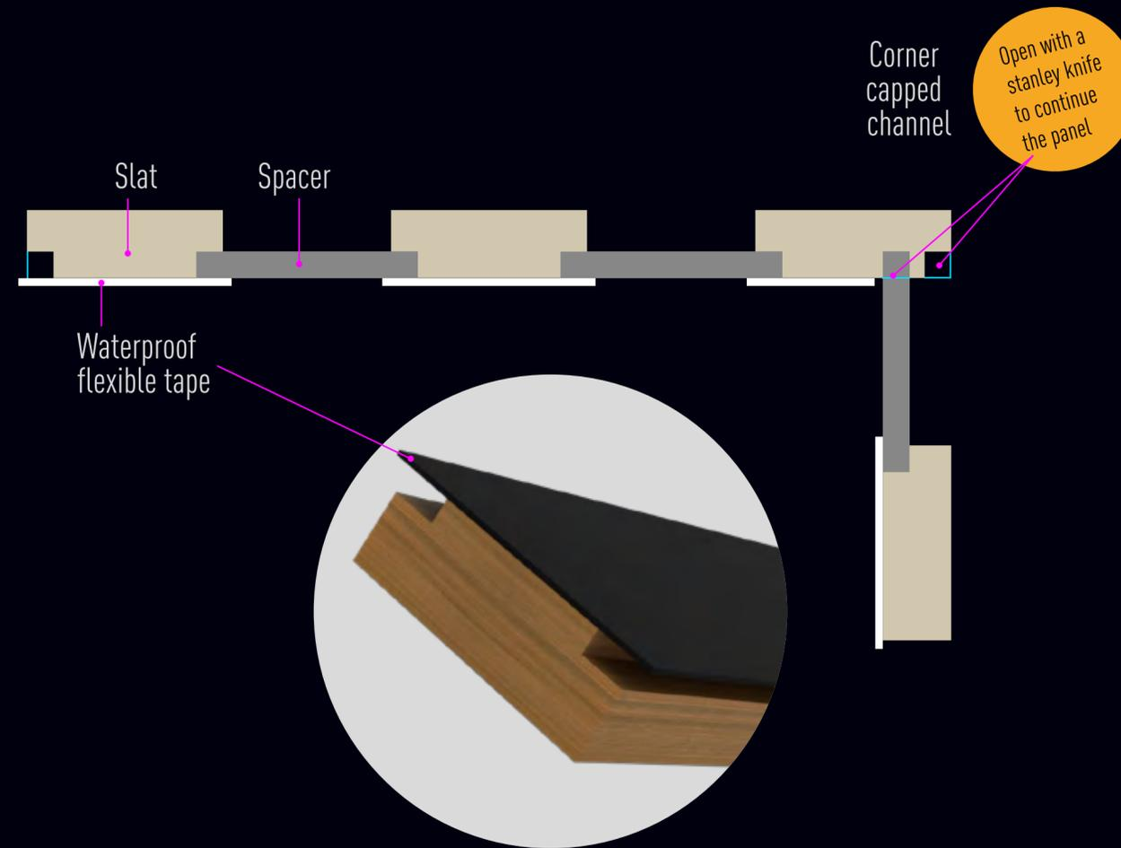
**FLEXIBLE TAPE + MDF + SPACER = FLEX SLATTED**
